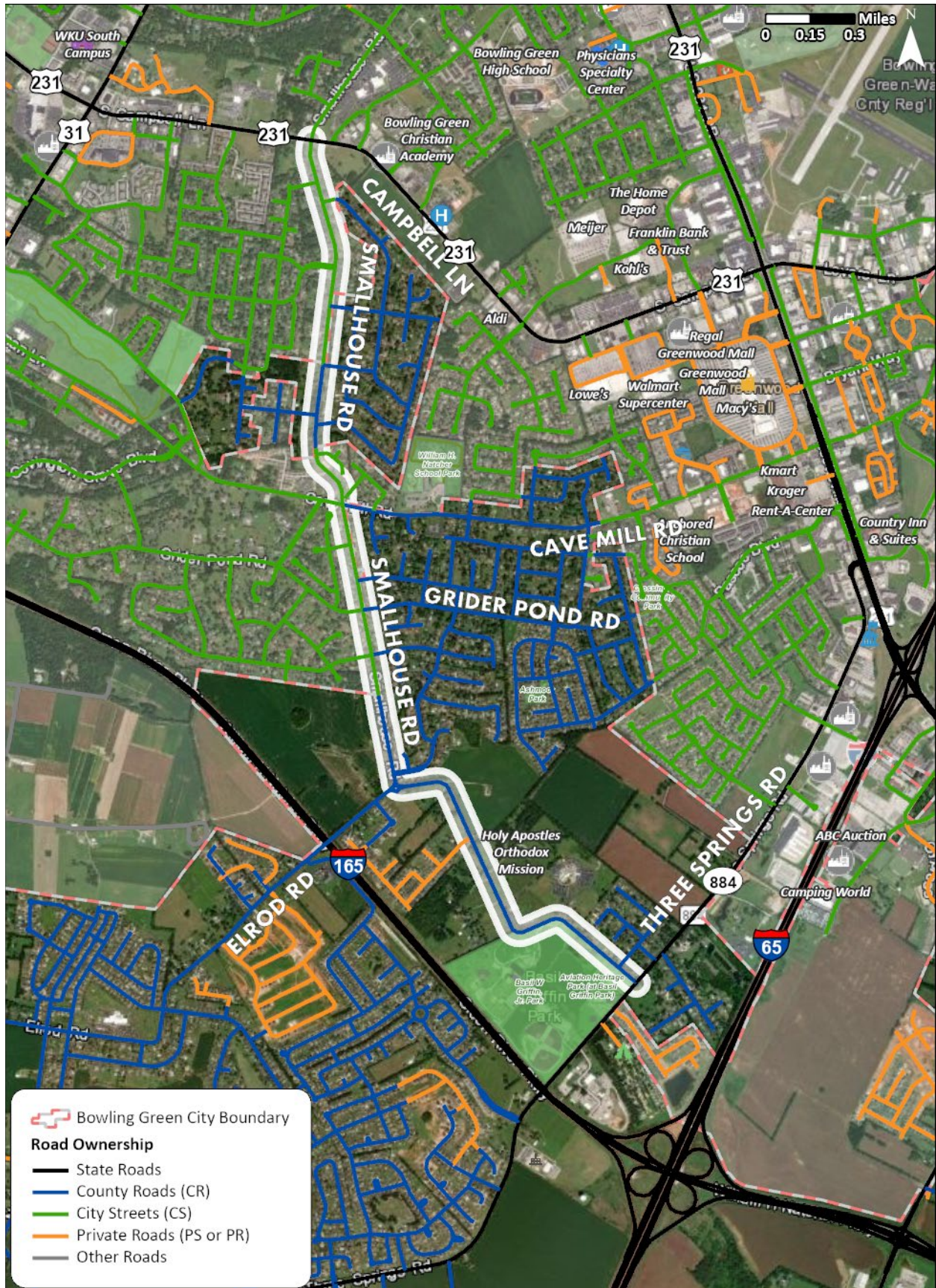
Figure 5. Ownership / Maintenance of Smallhouse Road
