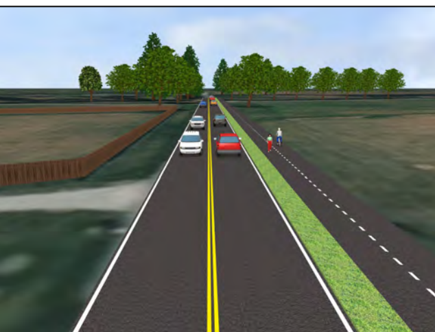
Shared-Use Path on One Side with Buffer (~36')
