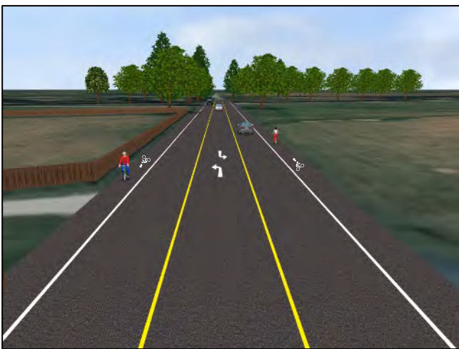
Center Turn Lane with Striped Bicycle Lanes (~44')
