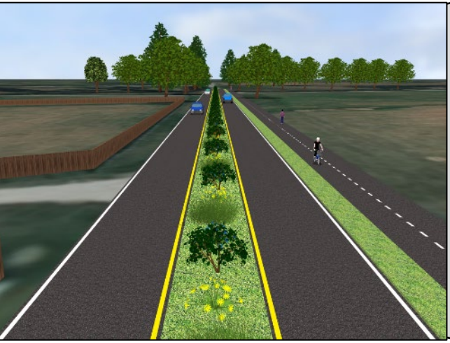
Center Median with Shared-Use Path on One Side with Buffer (~46')
