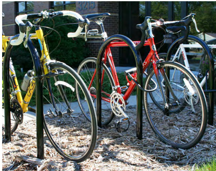
Below: This standard U- or hoop-rack is inexpensive and provides a secure option for bike parking.
